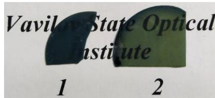
Figure 1 Photograph of ZnO:Ga (1) and ZnO:In (2) ceramic samples.
