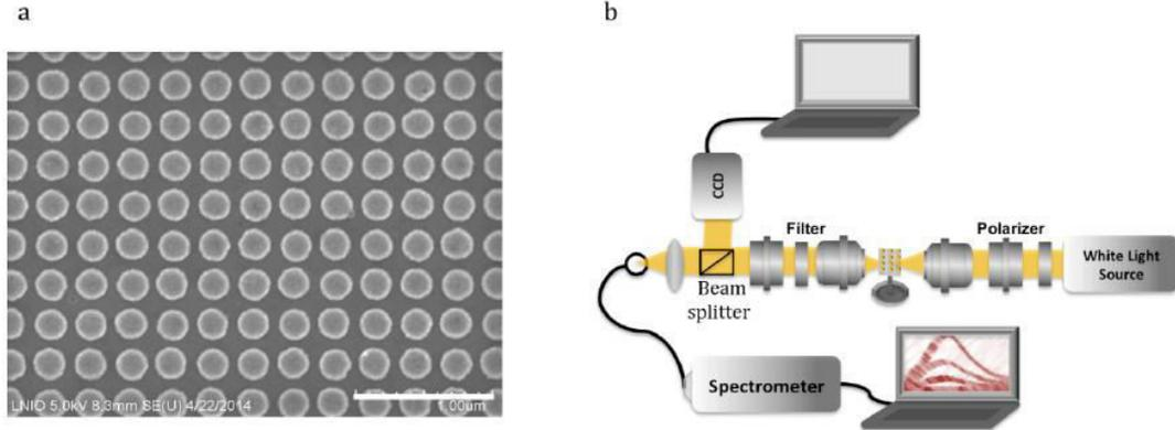
Figure 1: (a) SEM image of the grating of Au NPs, the scale bar is  $1\mu\text{m}$ . The experimental set up is presented in (b).
