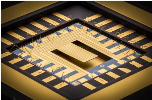
Figure 1: ScAlN based vibrational energy harvester.
