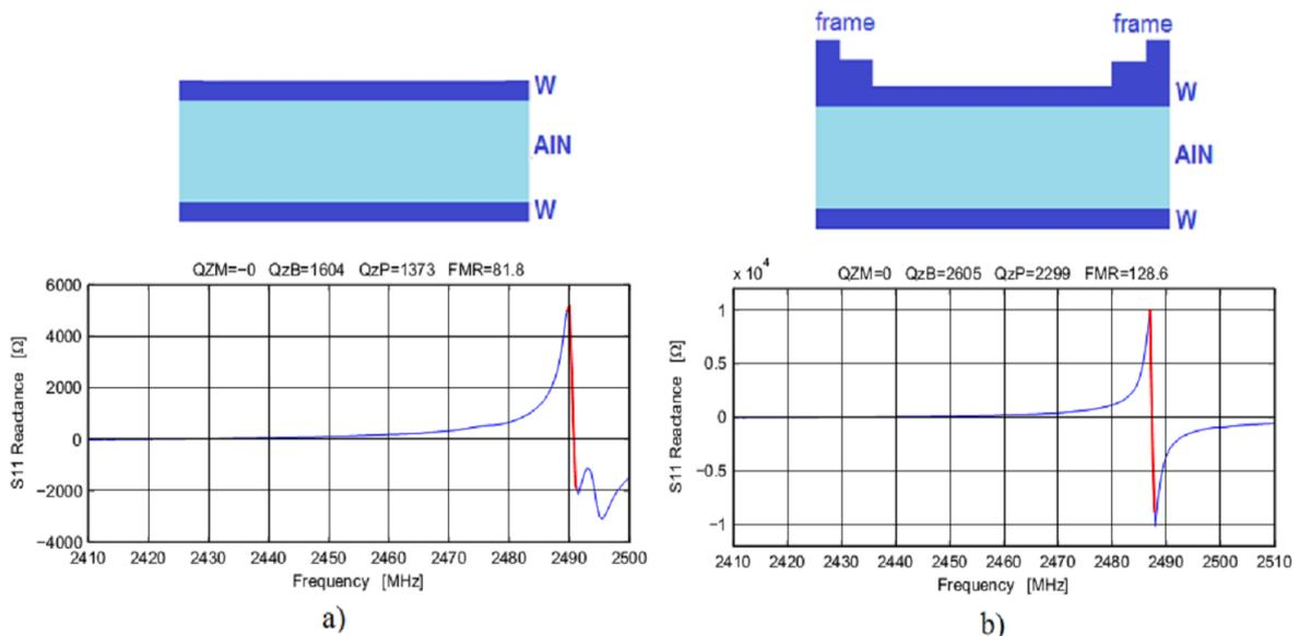
Fig. 1. 2D schematics and frequency responses of a traditional FBAR (a) and a frame-designed FBAR (b)
