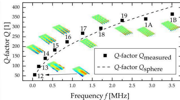
Figure 2: Q-factor of roof tile-shaped modes in deionized water.
