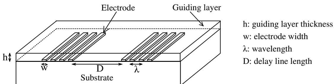
Figure 1: Schematics diagram of Love wave device
