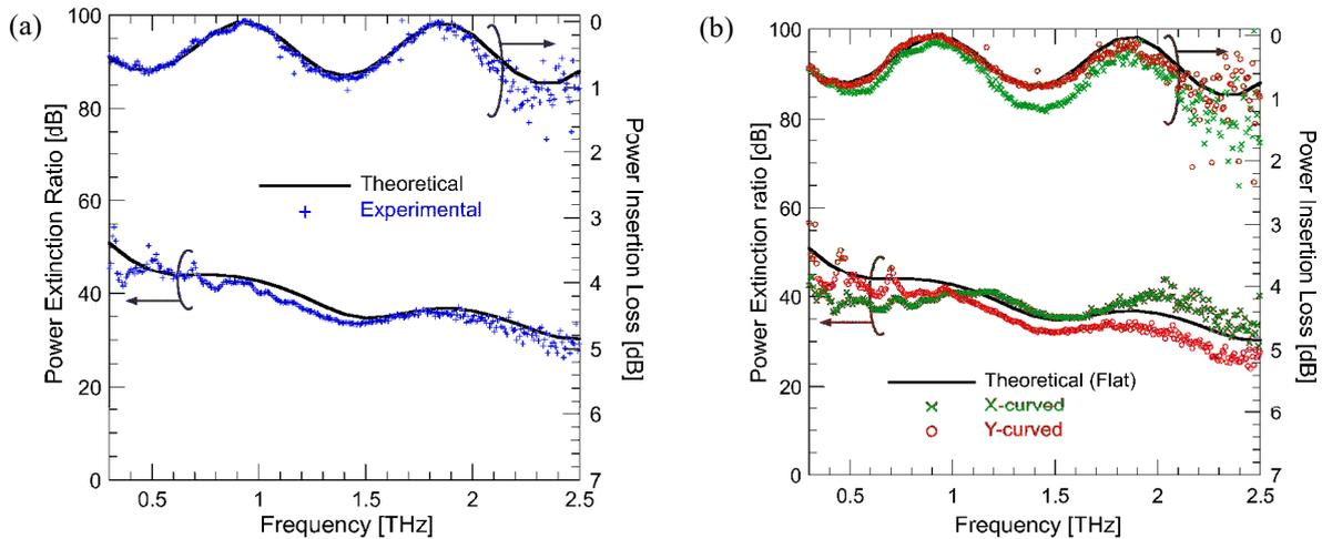
Figure 1: a) Comparison of experimental measurements and numerical results of the ER and IL for the THz WGP with a pitch of 10  $\mu\text{m}$  and a filling ratio of 68% for normal incidence. b) Experimental investigation of the ER and IL for the THz WGP in two bending configurations.
