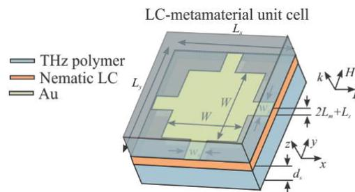
Figure 1: Fishnet Metamaterial unit cell
